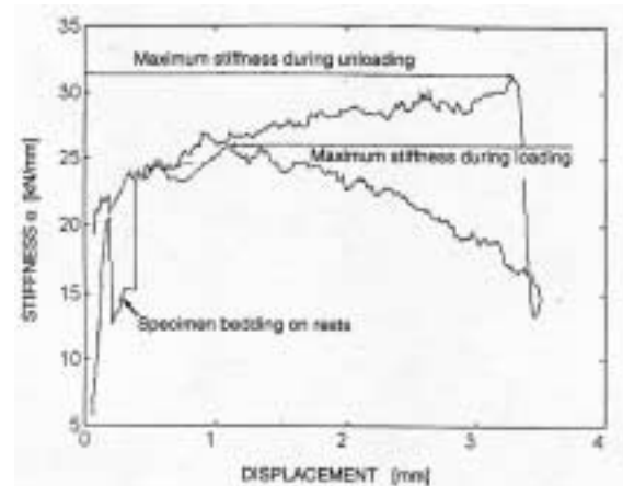
Fig.4 – Typical stiffness function during loading and unloading
